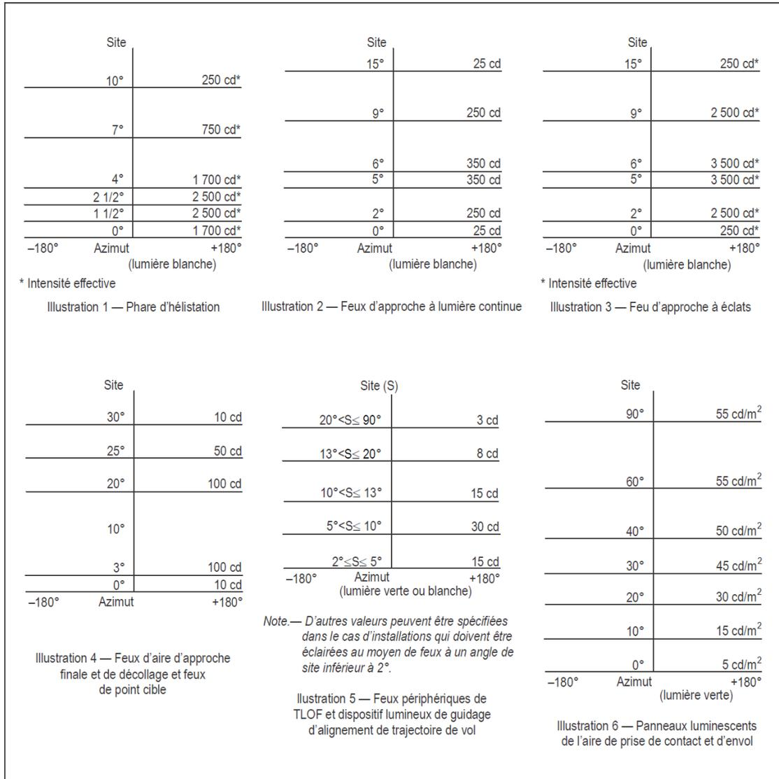
Figure 5-12. Diagrammes isocandelas
